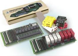
as the contact ratings are not exceeded. In addition, electromechanical relays are available in several "forms" (Form A, or Normally Open, Form B, or Normally Closed, and Form C, or a combination of Forms A and B) and a wide variety of pole configurations (SPDT, DPDT, etc.). This enables them to better serve as cross point and multiplexing switches as opposed to simple on/off devices.
