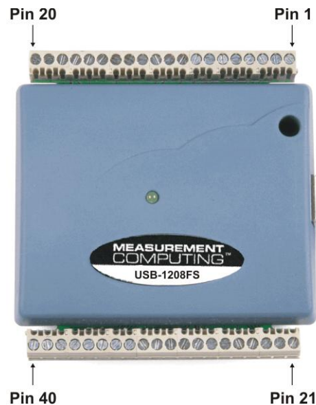
Figure 4. USB-1208FS Screw terminal pin numbers
