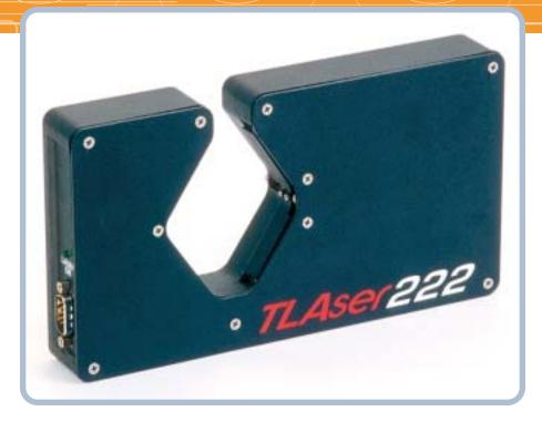
The TLAser222 gauge measures product diameter and position in two planes at right angles to each other—making it possible to check ovality and detect flaws continually using only one compact micrometer. LaserLinc's system design also offers the unique capability to measure multiple strands simultaneously with just one TLAser222 gauge.
