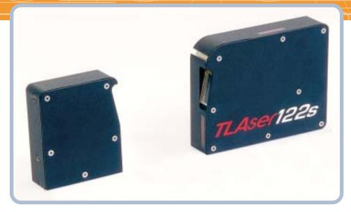
Except for its two-part housing, the single-axis TLAser122S Micrometer is nearly identical to the standard TLAser122 gauge. Separating the transmitter and receiver in their own respective units enables them to be mounted with a greater distance between them to make room for larger products and multiple assemblies.
