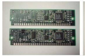
Front of compatibility modules; (top) TLAser—note: most chips not populated); (bottom) encoder—note: jumper in upper left.
