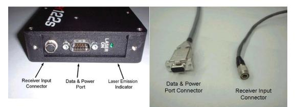
Receiver Input Connector—The round six-position connector is keyed and cannot be connected incorrectly. To connect, gently push while rotating connector until it 'snaps' in. To remove, grasp connector body and pull straight back.
