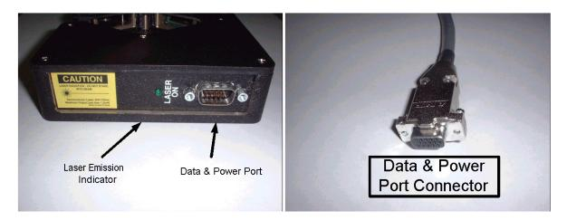
Power and Data Port—the D-style connector is keyed and cannot be connected incorrectly. DO NOT force the cable connector into the plug as damage may occur. Check the orientation if resistance is felt. The connector, if oriented correctly, will slide snugly into the socket. Jackscrews should be connected to prevent pullout. To remove, loosen jackscrews and grasp the metal plug housing and pull directly away from the scanner.
