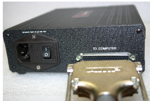
Figure 4. Remote Power Supply Box Connections
