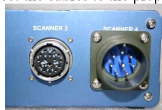
Figure 3. Zumbach Connection (on right) vs. Other Manufacturers'
