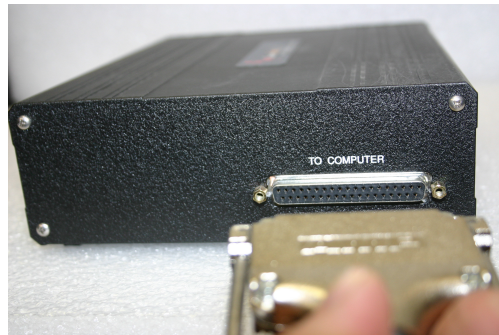
Figure 1. Plugging in the Cable Condenser Box
