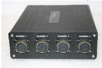
Figure 2. Cable Condenser- Power Supply Box - Gauge Connections
