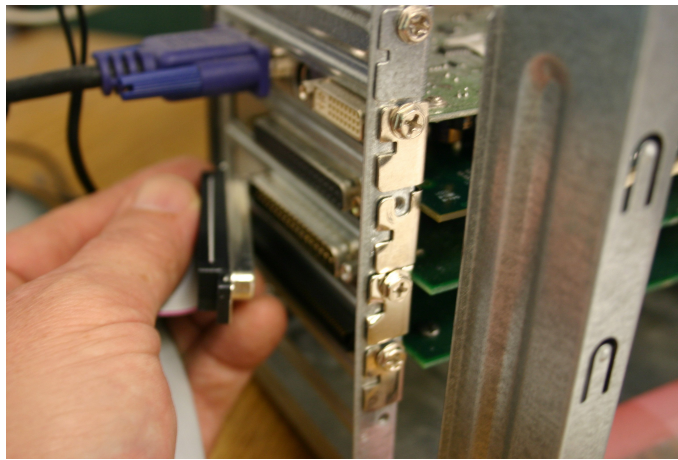
Figure 1. Plugging The T-Box into the CTR05 Card
