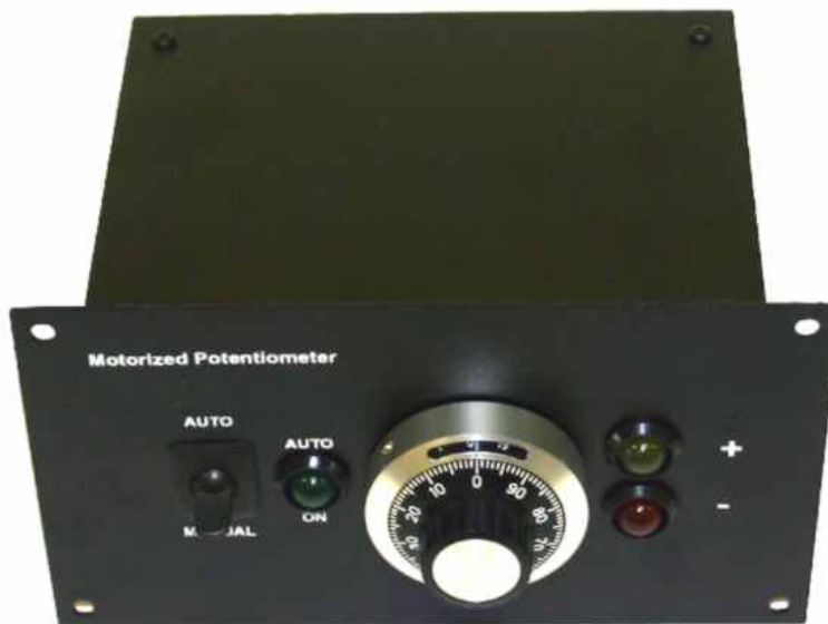
Figure 24. Motorized Potentiometer (MOP)—Front View
