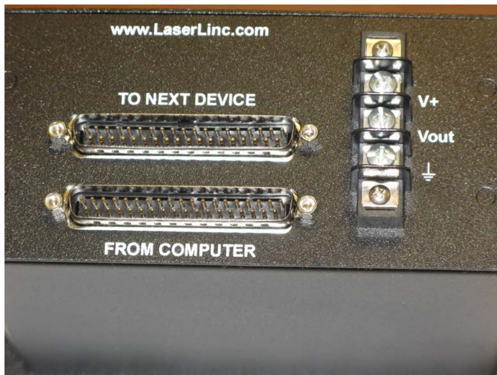
Figure 19. Motorized Potentiometer (MOP)—Rear View.
