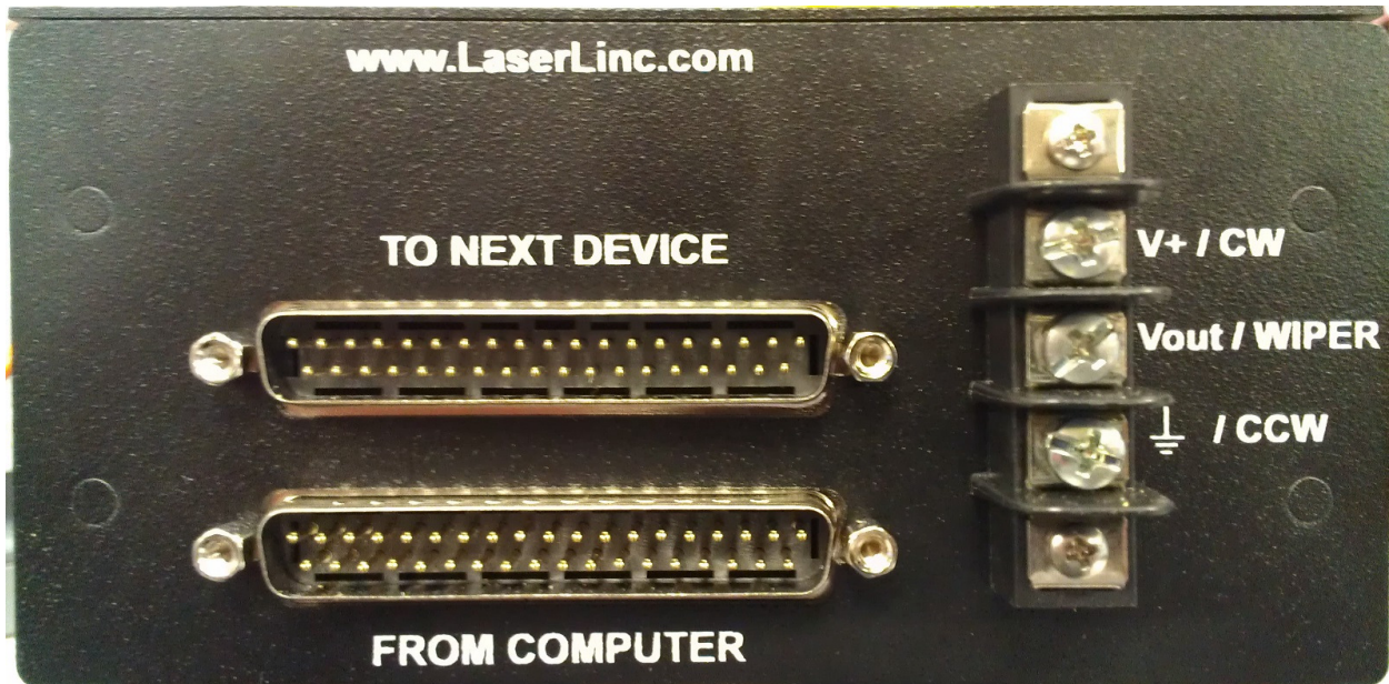
Figure 19. Motorized Potentiometer (MOP)—Rear View.
