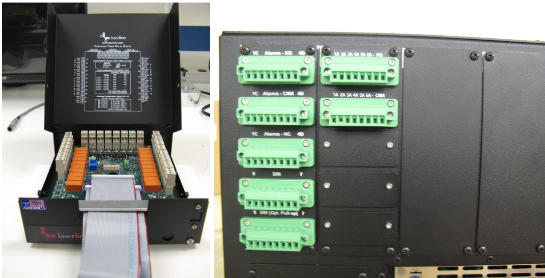
Figure 1. Enclosure Box Configuration (left), \mu Linc Configuration Terminal Blocks (right)
