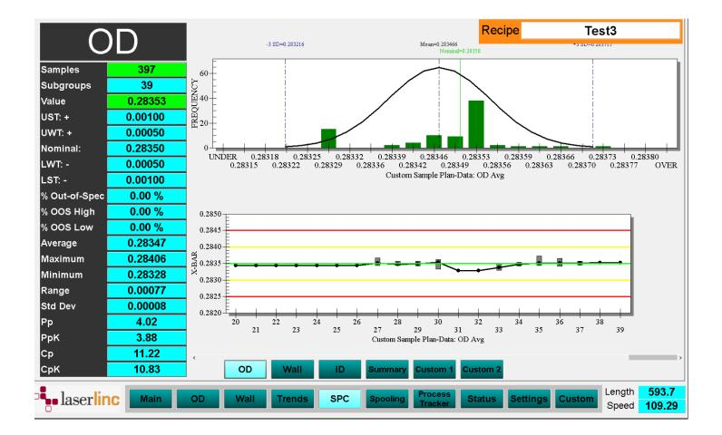
The SPC tabs are used to obtain statistical data about the outer diameter, wall thickness or inner diameter. Each tab shows advanced statistics, as well as a histogram and x-bar and range chart.
