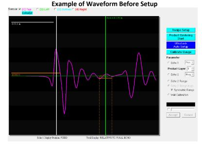
1. **Loading a Recipe**- The first step to setting up a run is to load a recipe. This can be done by clicking the "Recipe" button on the primary display and selecting the appropriate recipe.
